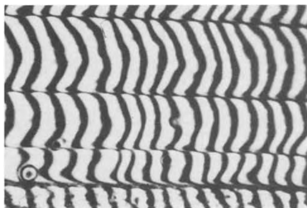
Fig. 4. Off-facet striations in space-grown InSb(Se); dual beam interferogram of etched, longitudinal section. Fringe contrast in space-grown section is much enhanced due to improved microhomogeneity. Magnification 140X.
