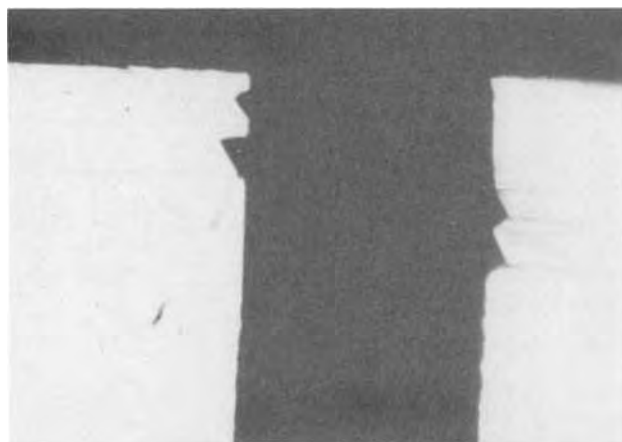
Fig. 8. Cross sections of etched heterostructure slices. The etched surface shown in (a, left) is a (011) plane. The etched surface of (b, right) is the (011) plane, which is perpendicular to the (011) plane of (a). The preferential etching is obtained with an etchant consisting of 0.3 mol/liter KI and 0.2 mol/liter \text{I}_2 ; the \text{pH} is 4. The etching time is 10 sec.
