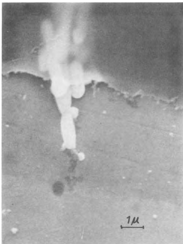
Fig. 6. Sulfide covered with reaction products. The reaction has proceeded under the lacquer causing detachment from the metal surface.
