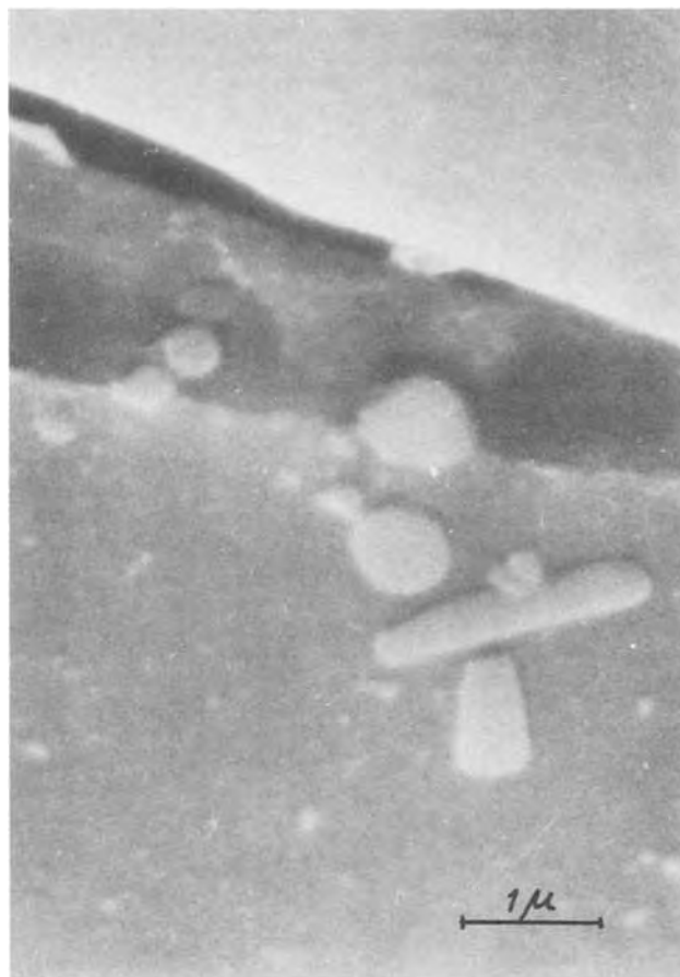
Fig. 3. Corrosion products around the initiation point; the light rods and spheres are manganese sulfides covered with reaction products.
