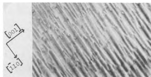
Fig. 4. Formation of ridge-type growth at 10 C/cm 2 at 20 mA/cm 2 on the (110) copper plane. 625 \times . (10 C/cm 2 = 3.6 \mu m).
