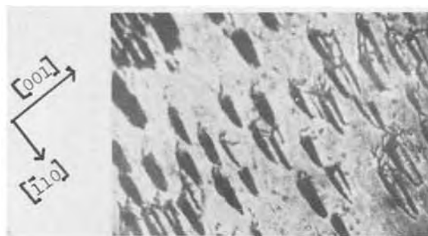
Fig. 3. Merging of rectangular pyramids at 8 C/cm 2 at 20 mA/cm 2 on the (110) copper plane. 625 \times .
