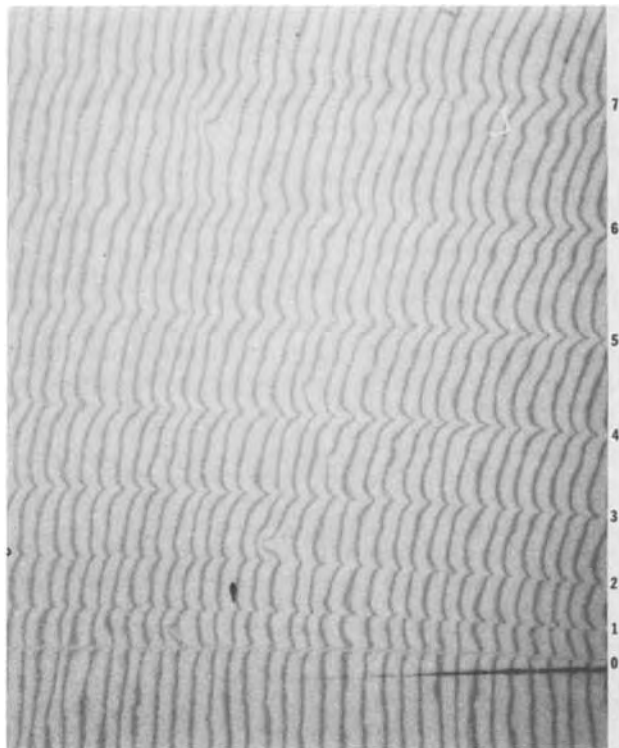
Fig. 3. Off-facet striations in space-grown InSb(Se); Tolanski multiple beam interferogram of etched, longitudinal section. Note the decreasing fringe deflection-peak sharpness with increasing order number of striations. Dark streak is fault in Fizeau plate. Magnification 100X.
