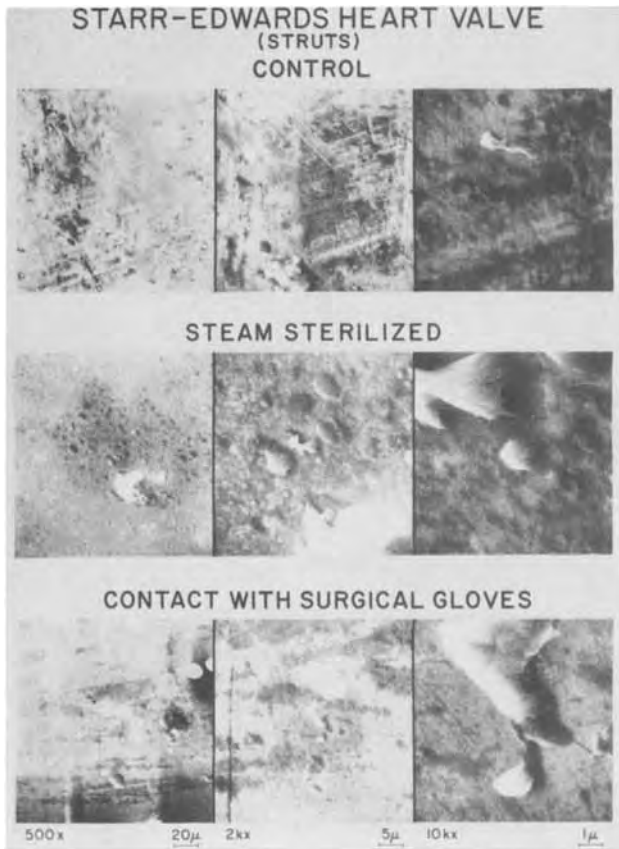
Fig. 11. Scanning electron microscopic (SEM) examination of a Stellite-21 Starr-Edwards heart valve showing the bare and contaminated surfaces.
