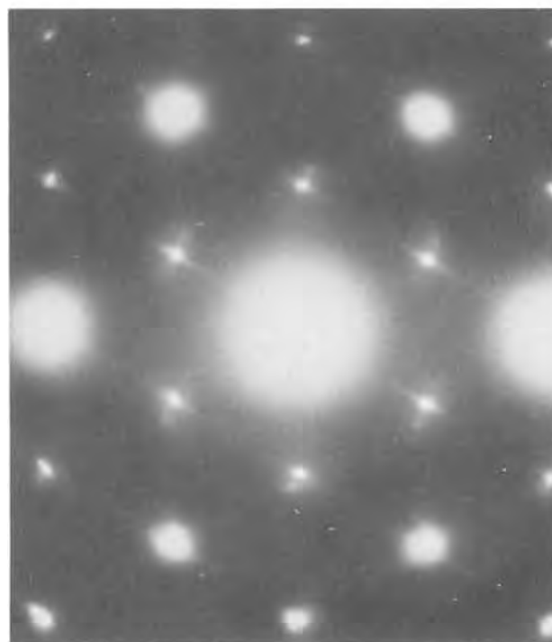
Fig. 3. TEM results for thin gold deposit on {111} substrate. (a, top) Bright-field image, original magnification 120,000 \times . (b, bottom) Selected-area diffraction pattern.
