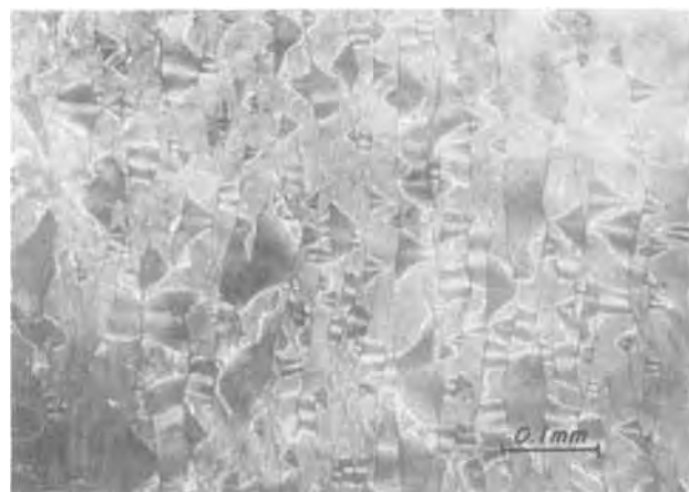
Fig. 15. 100V tantalum oxide film on chemically polished substrate subsequent to 0.45% strain. Tensile axis is horizontal. Random spacing of normal fracture lines.
