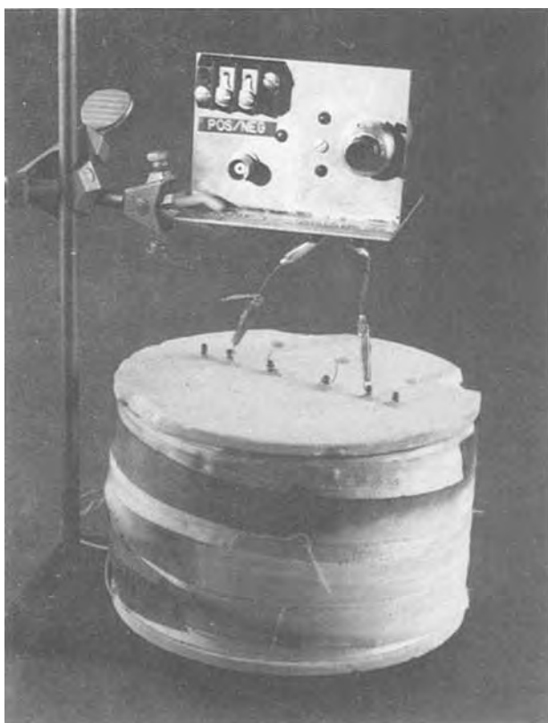
Fig. 2. Galvanostatic pulse generator and sample oven
