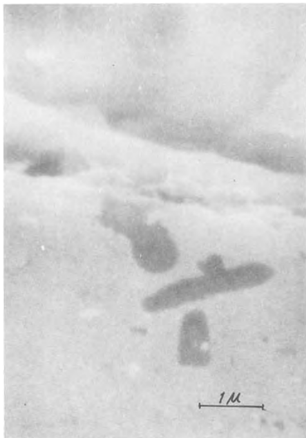
Fig. 4. Same area as in Fig. 3 after removal of the lacquer and wiping the surface with cotton wool. The dark areas represent manganese sulfides free from reaction products.
