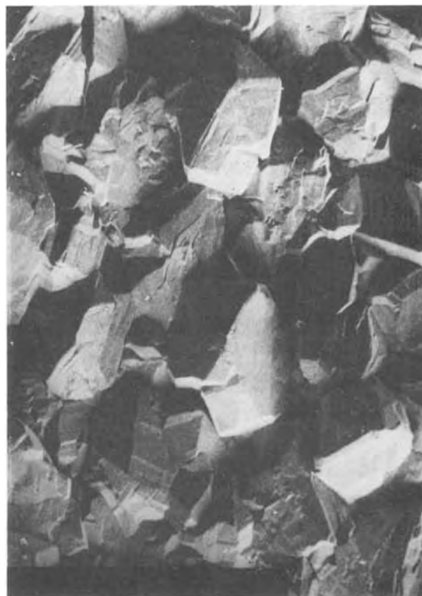
Fig. 9. Observation of the upper surface of a silver deposit obtained from a silver nitrate solution with thiourea (scanning microscope 100X).
