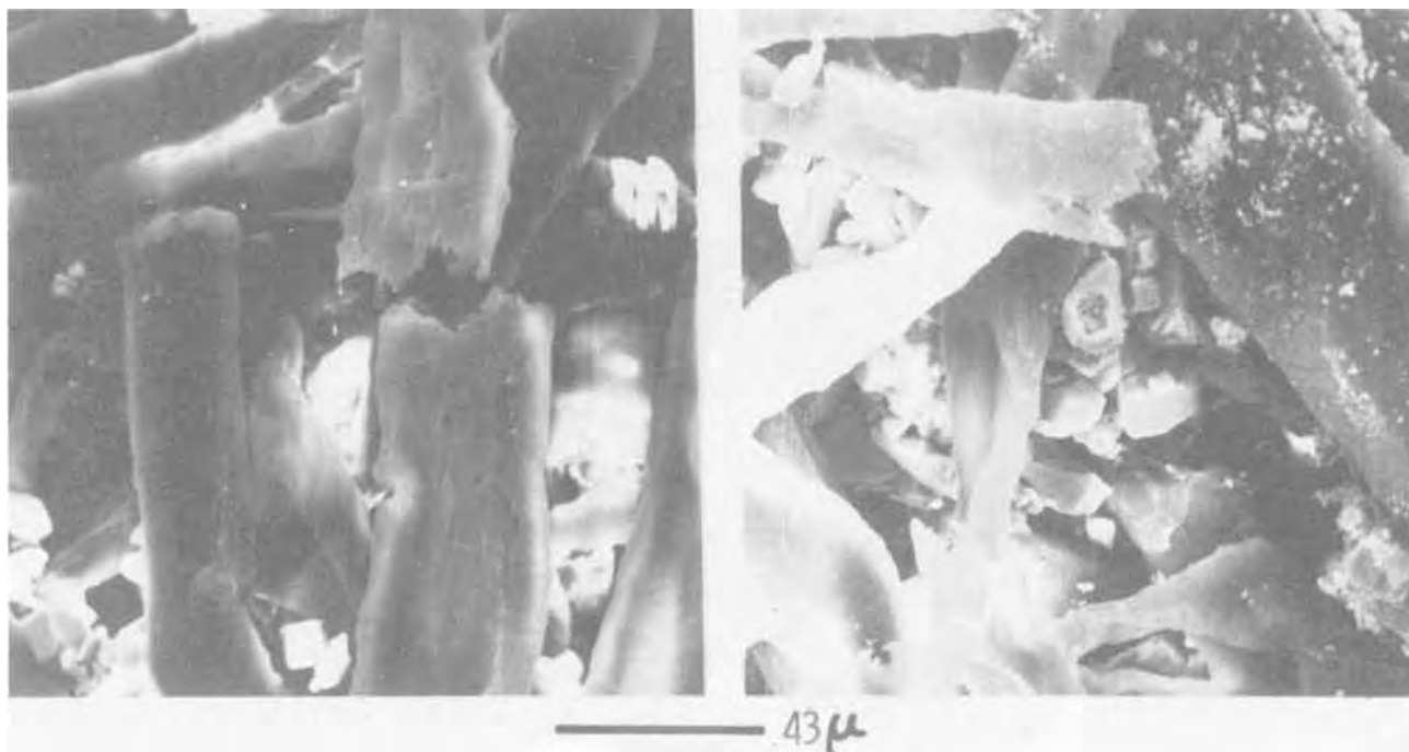
Fig. 13. Electron micrographs of brittle fractures. Because of the nature of the growth, it is clear there are compressive stresses in a direction perpendicular to the plane of the paper.
