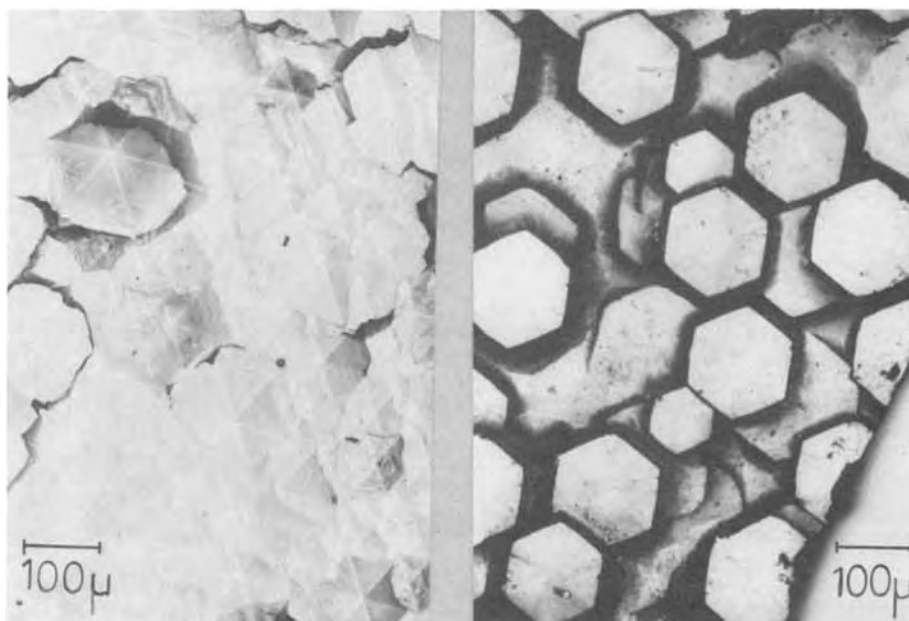
Fig. 6. Two kinds of as-grown surfaces of the Zn-doped GaN.
