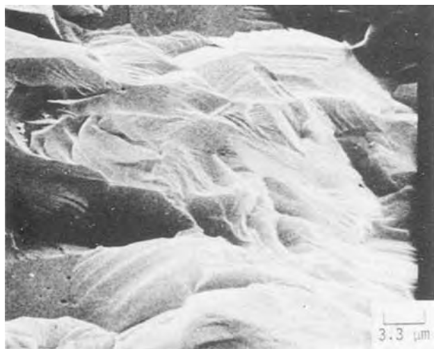
Fig. 1. SEM photograph of a fractured surface of a typical pre-test AlN sample.
