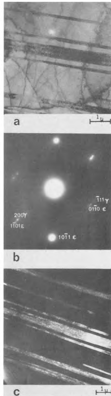
Fig. 12. \epsilon -hexagonal martensite bands in AISI 304 L steel deformed 15% by tensile stress at room temperature: (a) bright-field image; (b) electron diffraction pattern, [011]_{\gamma} and [1011]_{\epsilon} zone axes; (c) dark-field image obtained by 1011_{\epsilon} -reflection.
