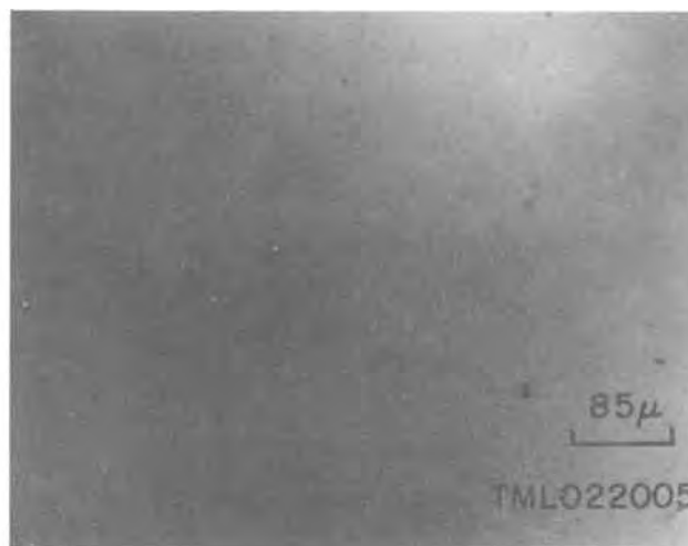
Fig. 3. Photomicrograph (Nomarski phase contrast) of a layer grown at 735°C on a substrate that had undergone a porous oxide-HCl treatment in addition to standard cleaning. Growth parameters were unchanged from that shown in Fig. 2. The improvement in the wetting is remarkable.
