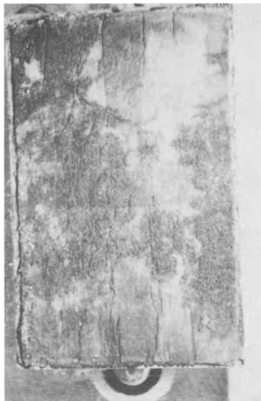
Fig. 6. Photograph of used zinc electrode from cell A. The electrode was discharged before removal from the cell. Total charge delivered to the electrode during cell operation was approximately 219 A-hr. The distribution of unconsumed, metallic zinc appears as dark, rough appearing areas.
