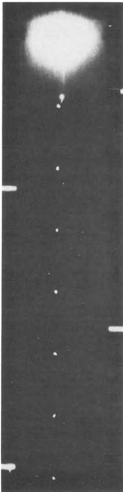
Fig. 3. Initial segment of a typical film strip of a carbon particle burning in pure oxygen at 1 atm pressure. Initial size of the particle was about 100 \times 130 \times 130 \mu\text{m} . Magnification on the 1.6 cm wide film is 2.32. Time runs top to bottom. Initial bright region represents the laser pulse. Timing marks on the left edge are spaced 1 msec apart.
