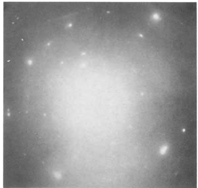
Fig. 6. Transmission electron diffraction pattern of reactive plasma BN deposited on (111) Si substrate.
