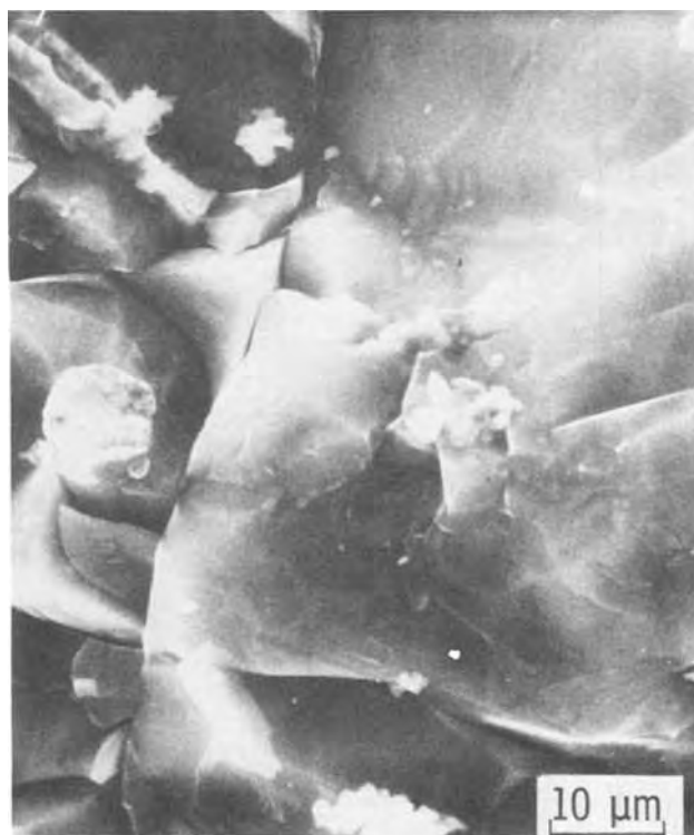
Fig. 6. Scanning electron microscope photograph of the solidified melt of 72.4 m/o Li-Si alloy after annealing at 925^\circ\text{K} for 14.5 ksec showing a single phase of the compound \text{Li}_{21}\text{Si}_8 .
