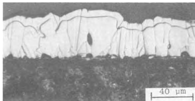
Fig. 8. Mechanically polished and chemically etched surface of the vertical cross section of a polycrystalline silicon solar cell deposited on a graphite substrate by using a hydrogen-trichlorosilane-hydrogen chloride mixture (the n + -layer was removed by etching).
