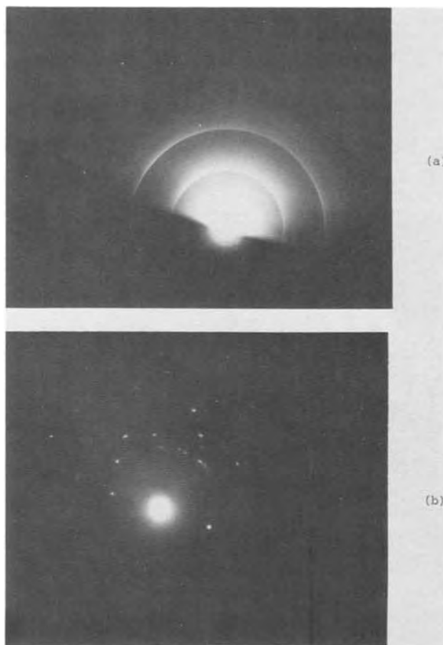
Fig. 3. (a) Reflection electron diffraction pattern of Pfizer compression-annealed pyrolytic graphite. (b) Transmission electron diffraction pattern of reactive plasma BN deposited on Pfizer compression-annealed pyrolytic graphite.
