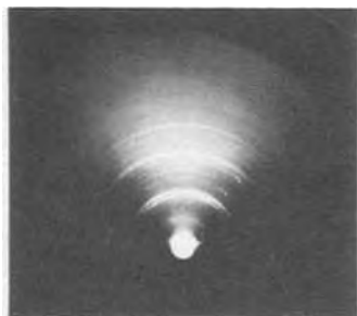
Fig. 1. Electron reflection pattern observed from the blacked surface of copper which is used practically as a sunshine absorber. The reflections correspond to those of monoclinic \text{CuO} . The (020) reflection shows a preferred orientation in relation to the substrate face. Wavelength of the electrons = 0.0304\text{\AA} . Distance between the specimen and the screen = 50 cm.
