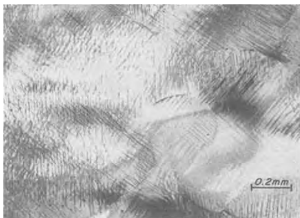
Fig. 5. 35V aluminum oxide film and substrate subsequent to 10% strain. Tensile axis is horizontal. Normal film failure followed by failure at substrate slip lines.
