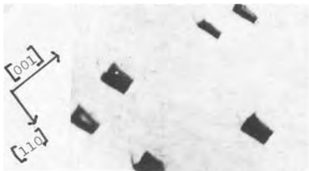
Fig. 1. Formation of rectangular pyramids at 2 C/cm 2 at 20 mA/cm 2 on the (110) copper plane. 625 \times .
