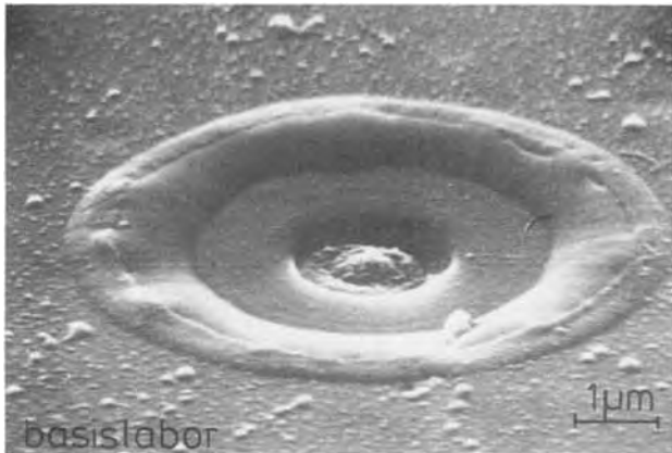
Fig. 3. Scanning electron micrograph of area in an Al-SiO 2 -Si capacitor where self-healing breakdown took place.
