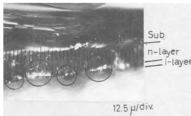
Fig. 4. Observation of the light occurrence (encircled) at the cleaved surface with a forward bias. The In contact over the i-layer surface is out of focus in the photograph.
