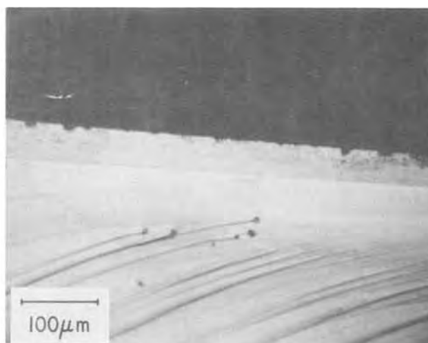
Fig. 5. Cleaved substrate showing epitaxial layer grown at 480^\circ\text{C} from a charge of \text{Pb}_{0.791}\text{Sn}_{0.211}\text{Te} at 590^\circ\text{C} . 160X magnification.
