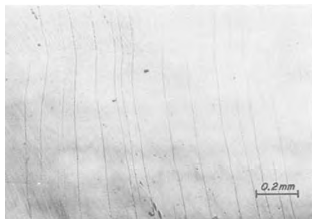
Fig. 4. 50V aluminum oxide film and substrate subsequent to 1.2% strain. Tensile axis is horizontal. Normal film fracture.
