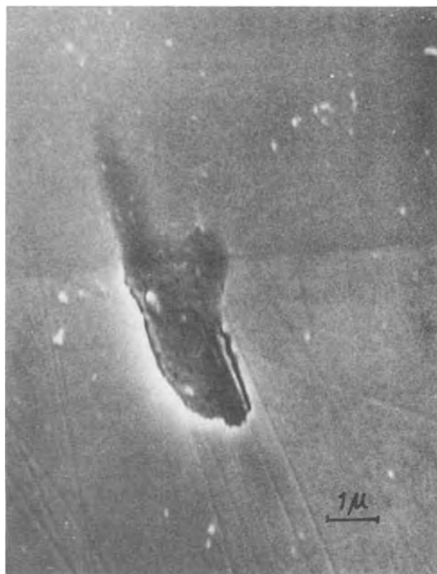
Fig. 5. Inclusion situated at the junction between the lacquer and the free metal surface. Part of the inclusion faintly visible under the lacquer. The inclusion is preferentially dissolved along the sulfide-metal interface.
