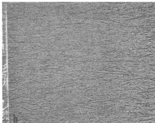
Fig. 6. Microstructures of cobalt deposits prepared from (a) CoSO_4-V_2O_5 plating solution, insoluble anode is used and (b) CoSO_4 plating solution, soluble anode is used. Plating conditions are reported in Table II. 1000 \times magnification.
