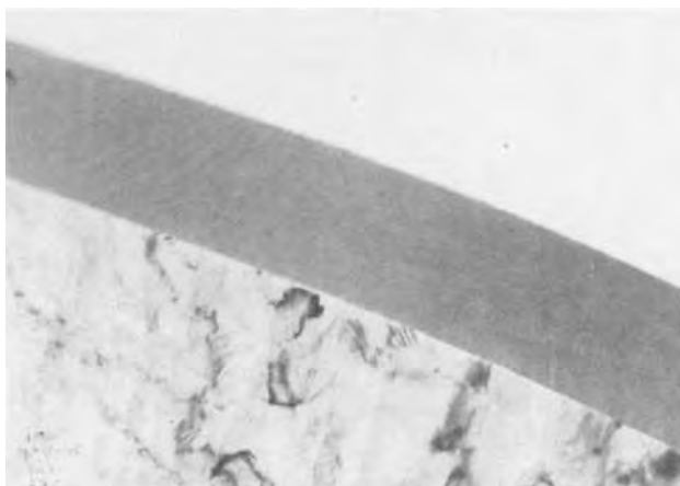
Fig. 11. Transmission electron micrograph of a 500Å thick cross-section of an anodized Al sample. The lower part is the metal. The oxide layer is about 2600Å thick.
