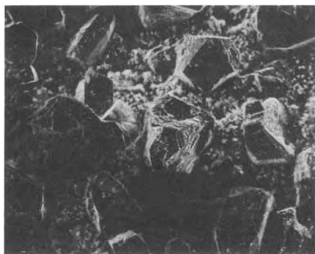
Fig. 3. 300X SEM photograph of zinc deposited from ZnCl 2 -NaCl-KCl eutectic.
