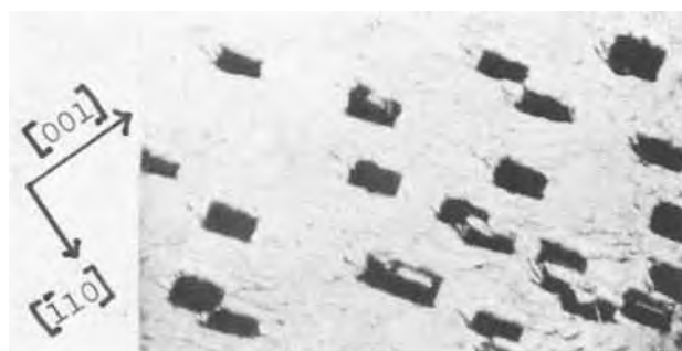
Fig. 2. More number of rectangular pyramids at 4 C/cm 2 at 20 mA/cm 2 on the (110) copper plane. 625 \times .
