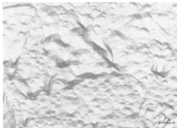
Fig. 12. Transmission electron micrograph of anodic tantalum oxide film formed on chemically polished substrate at 50V for 3 hr.
