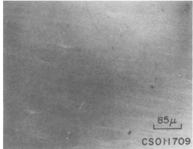
Fig. 4. Steps caused by a fast growth rate. This particular layer is about 0.2\mu thick and grown at 780^\circ\text{C} . The growth parameters are: supercooling \Delta T = 3^\circ\text{C} , linear cooling rate \alpha = 1^\circ\text{C}/\text{min} , and the growth time t = 15 sec.
