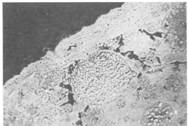
Fig. 3. Scanning electron micrograph of selectively amalgamated spherical alloy.
