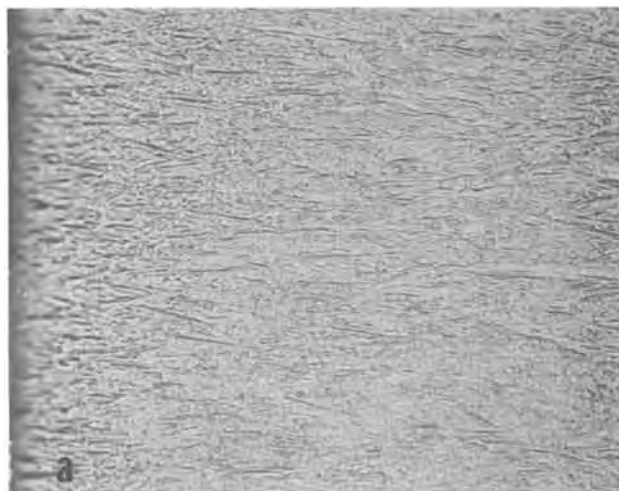
Fig. 6. Microstructures of cobalt deposits prepared from (a) CoSO_4-V_2O_5 plating solution, insoluble anode is used and (b) CoSO_4 plating solution, soluble anode is used. Plating conditions are reported in Table II. 1000 \times magnification.
