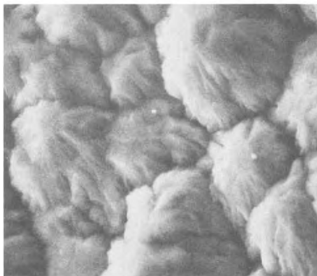
Fig. 4. SEM pictures of CdS on Cd 2 SnO 4 /silica substrate. Lower: as deposited. Upper: after 5 sec etch in 55% HCl solution at 40^\circ\text{C} . Width of field = 35 \mu\text{m} .
