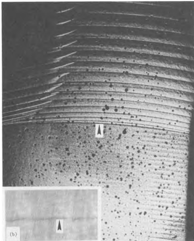
Fig. 1. Etched (111)A longitudinal section of InSb(Se) single crystal (sample E3-SL4). Arrow indicates demarcation between Czochralski-grown seed at bottom with rotational striations and space-grown section. (111)B solid-liquid interface facet striations at upper left, off-facet striations at upper right. Etch pits due to In-dislocations. Magnification approximately 17X. Inset (b) Melt-back interface, 125X.
