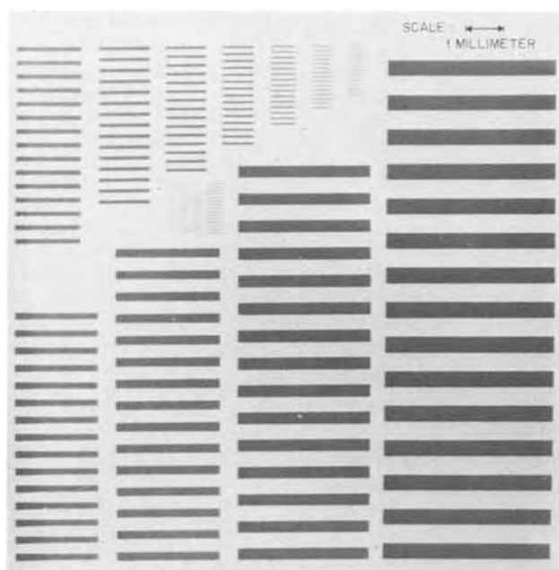
Fig. 12. A GaAs sample with deposited Ealing test pattern after anodization at 55V in water of pH = 2.5 and after removal of the photoresist. The oxidized areas are dark; original magnification was approximately 30X.
