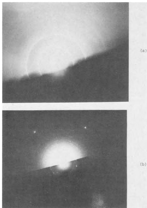
Fig. 2. (a) Reflection electron diffraction pattern of CVD BN deposited on Supertemp graphite substrate. (b) Reflection electron diffraction pattern of high temperature reactive plasma BN deposited on Supertemp graphite substrate.
